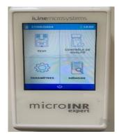
Select QC then EQA Test. Insert the test chip and wait for the countdown.
